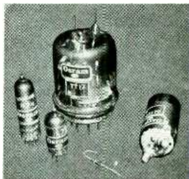
Group of Osram valves including the TT17, L77, N78, DET20 and a Germanium crystal.
