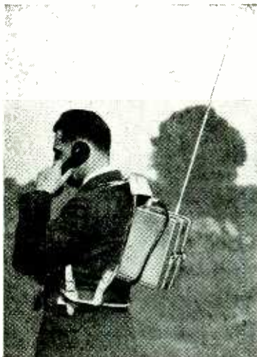
Marconi walkie-talkie (Type H19) as used by one of the airport staff.
